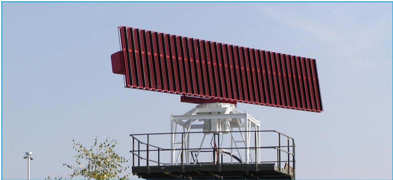
**MSSR-1 – Monopulse Secondary Surveillance Radar developed by ELDIS Pardubice, s.r.o. – is a fully modular system, which meets or exceeds ICAO and MARK X recommendations and standards and allows extension according to increasing needs of the customer. Individual modules of the equipment can be used either in new or in older MSSR systems.**
